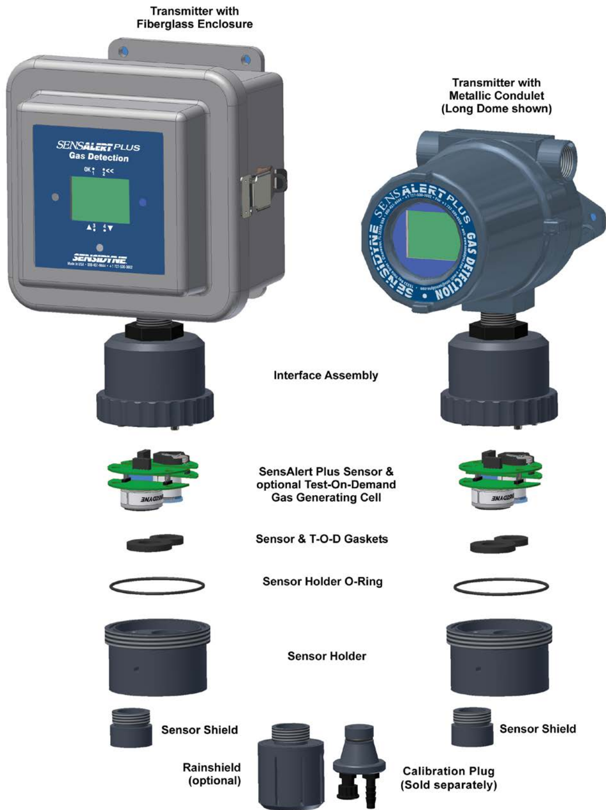
Figure 1-1 SensAlert Plus Transmitter Components
